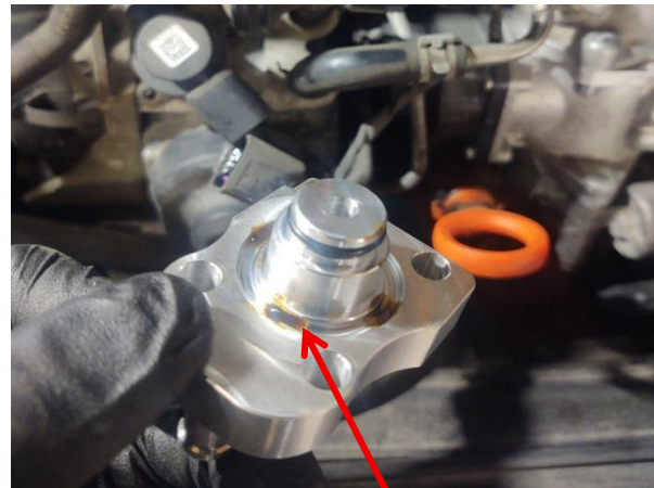
Grease dabs in large O-ring groove
