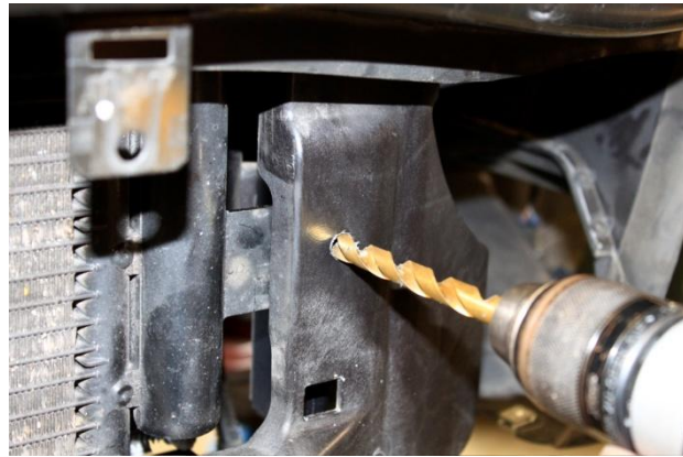
17. Attach both left and right side intercooler mounts into existing square holes in radiator core support, then lock down, now drill 1/4" thru core.
