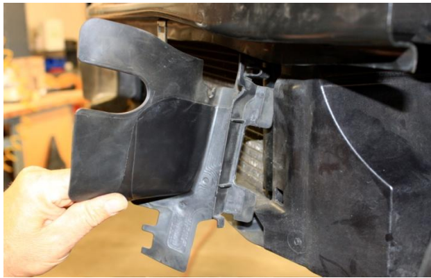
10. Unclip and remove the (2) radiator air deflectors.
