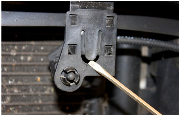
11. Remove plastic outside air temp mount from steel bumper then remove sensor from plastic mount.
