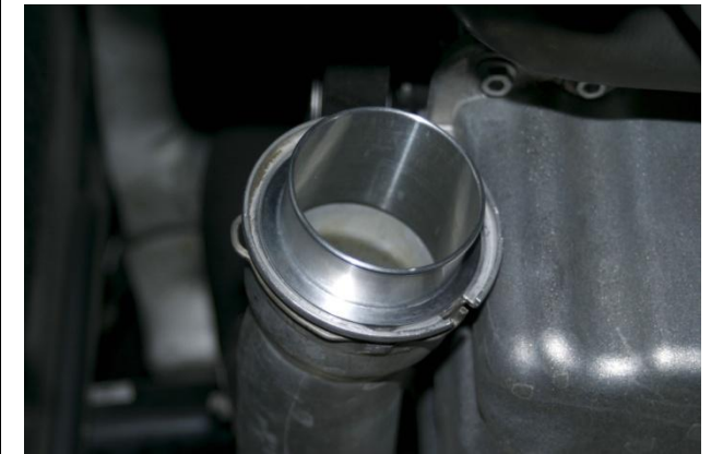
27. Install NEUSPEED billet hose coupling into turbo discharge pipe. Make sure clip locks onto billet adapter.
