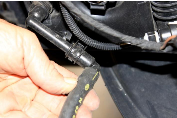
9. If equipped, disconnect headlight washer hose connection on the passenger side. NOTE: Cap or plug washer hose to prevent fluid loss from reservoir. Remove bumper cover and Styrofoam crash support.
