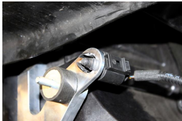
21. Install outside air temp sensor into hole in billet intercooler mount.
