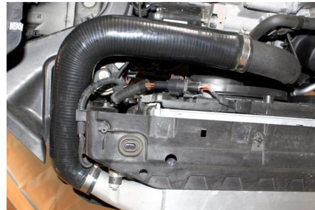
24. Install and tighten supplied driver side intercooler hose and clamps as pictured. NOTE: Clamp screw goes to back side of intercooler.
