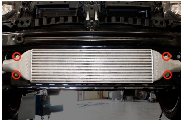
22. Mount intercooler core to vehicle using the supplied (4) 6mm hex flange nuts.
