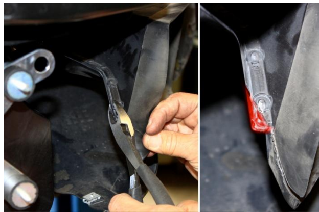
23. GOLF R ONLY: Cut off inside corner from plastic air duct for transmission.
