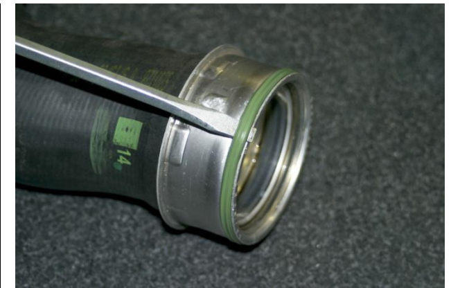
25. Carefully remove seal from passenger side factory intercooler hose.
