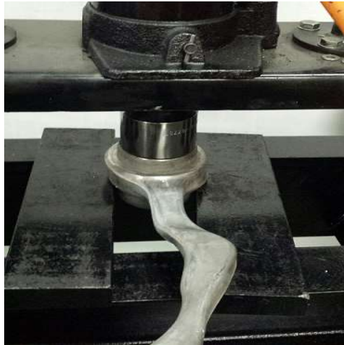
An alternate view of pressing the bushing out.
