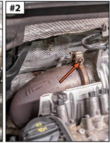
Step 8: T30 Torx, 7mm Socket & Torque Wrench
