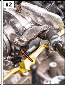
Step 10: M8 Triple Square, 10mm Socket & Torque Wrench
