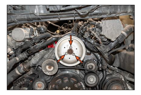
M10 Triple Square Socket & Torque Wrench Step 6:
