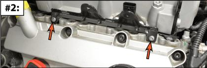
16mm Socket & Ratchet, 3/16" Drill Bit Step 16:
