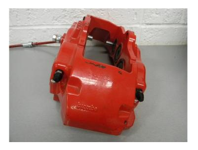
4. Install the transfer line onto the holes on the top of the caliper where the bleeder screws were removed. Tighten until snug, DO NOT OVER TIGHTEN to avoid stripping the aluminum threaded hole.
