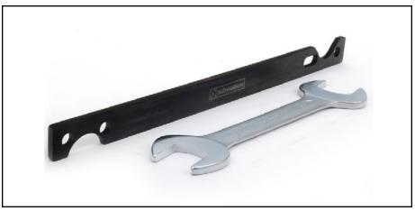
The BMW fan clutch tools are very helpful for removing the fan/clutch. The wrench fits the large nut that holds the fan/clutch to the water pump and the holding fixture will lock onto two of the water pump bolts so you can hold it stationary to break the fan loose.
