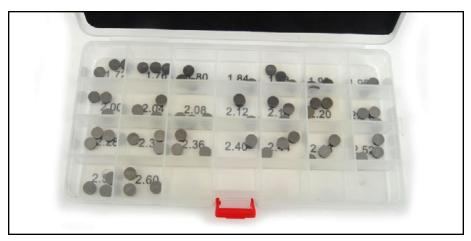
These shims are a must-have for the valve adjustment
