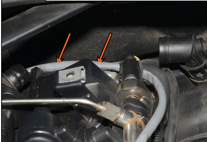
#3: Locate the two T30 rear inlet mounting screws, remove the rear inlet from the engine bay
