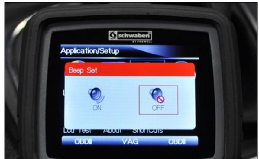
Once you select on or off and press the **Enter** key, the scanner will return to the "Setup" screen.
