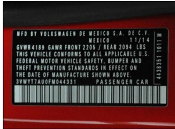
The door jamb ID plate is located in the lower rear area of the LH door jamb. The most important piece of information here is the build date, and the VIN is also located on this tag.
