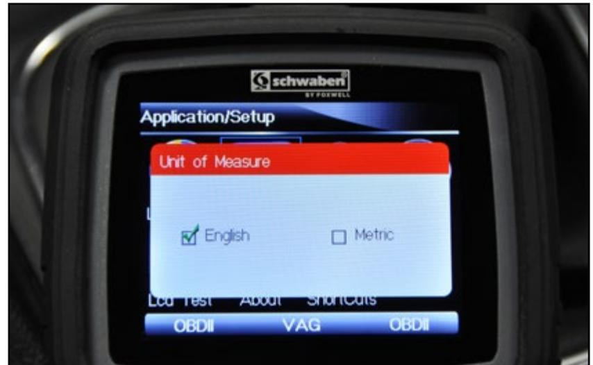
Once you select a unit of measure and press the **Enter** key, the scanner will return to the "Setup" screen.
