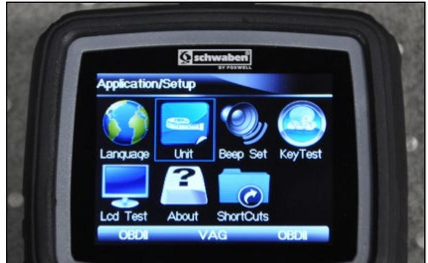
From the "Unit of Measure" screen, use the **Arrow** keys to select the unit of measure, then press the **Enter** key.
