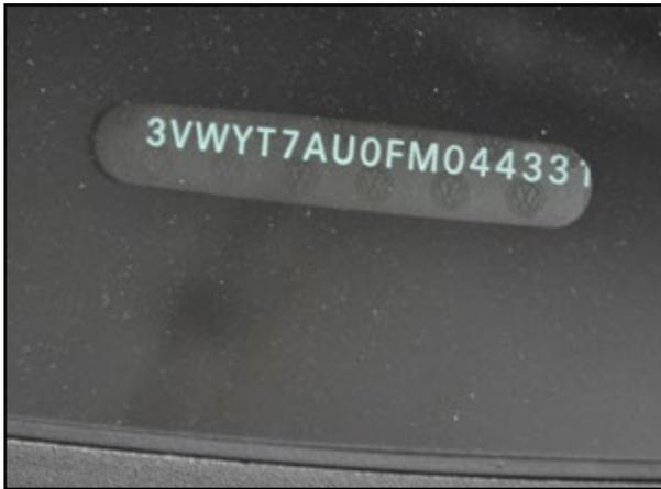
The windshield VIN plate is visible at the base of the windshield on the LH side. The VIN is located on the other ID tags as well but in many cases it is easiest to read here.
