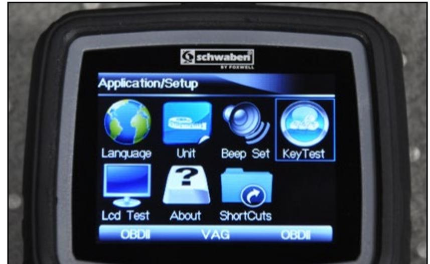
On the "Key Test" screen, press any key and the icon on the screen will be highlighted, indicating that the key is recognized and working properly.
