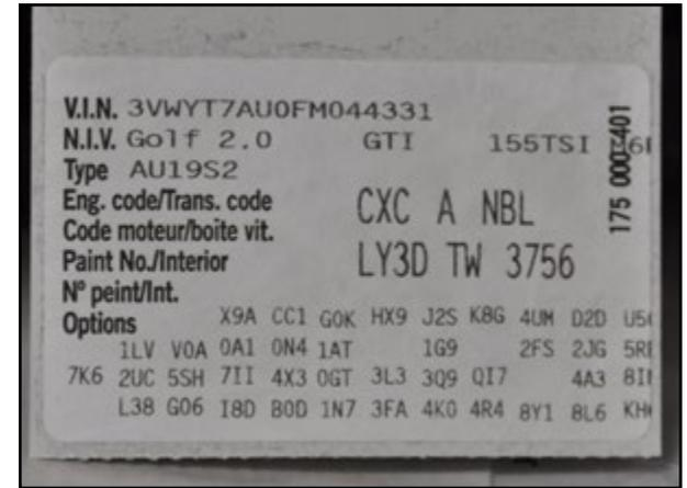
The service ID label is generally located in the trunk or spare tire area. It may be on the trunk lid, spare tire cover, or even on a rear shock tower. You may have to look around a bit to find it. This label will contain sales type, engine code, and transmission code.
