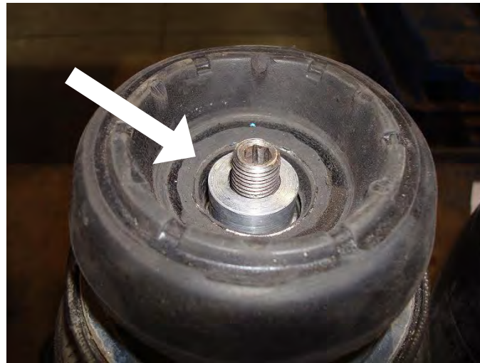
Rubber removed from VR6 mount
