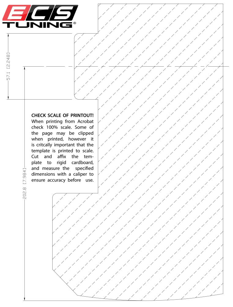
Wheel Clearance Template - VW MKV/VI - ECS Stage 5
