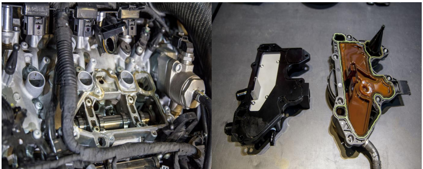
Step 4- Remove the OEM "PCV Plate" using T30 torx driver
