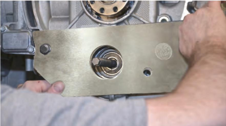
**Bearing extraction using conventional method with IMS Pro Tool Kit is now complete. Proceed to step 16.**
