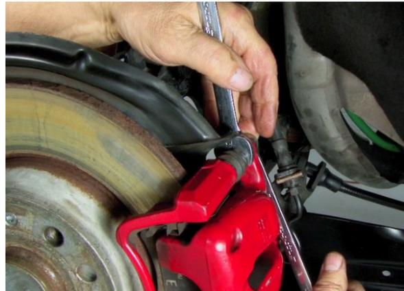
Remove the lower caliper-to-slide pin bolt the same way.
