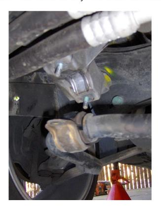
Draw a circle around the 13MM bolt where the mount is held onto the bracket. Also mark where the nub on the mount is that pokes through the bracket. This will help you align the new mount. Unscrew the 13MM nut holding the mount on the bottom.
