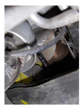
Unscrew the top nut on the driver side mount. You have a clear shot at it from the top. Here is the driver side mount from the top:
