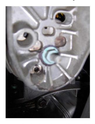
Now, unbolt the motor mount bracket from the car. Three 18MM bolts hold it on. You should have these removed from the car:
