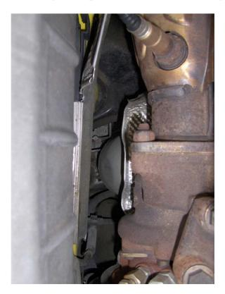
You can either remove the airbox to get to the top bolt, or do what I did, and get at it from under the car.
