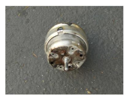
Toss your old mounts, and install the new ones using the old brackets, nuts, and bolts. Start the car with the mounts tightened slightly, and then let them settle into place and tighten them to spec.
