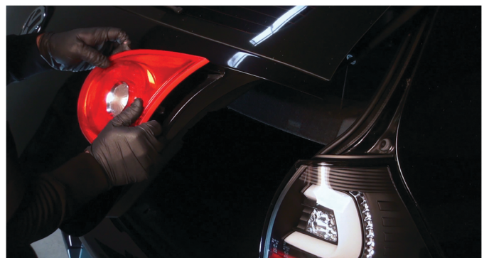
16) Unseat and remove the inner tail light.
