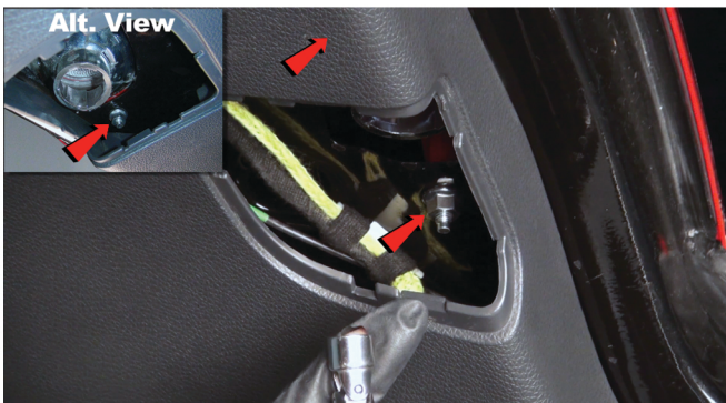
15) Remove [2x] 10mm nuts securing the inner tail light to the body.
