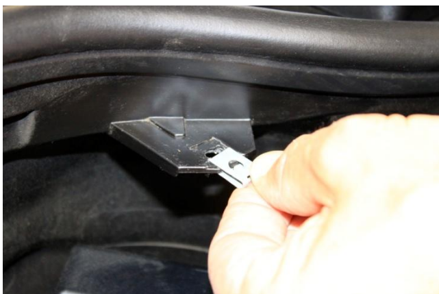
5. Remove and discard metal screw clip.
