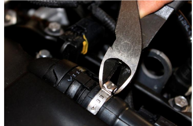
10. Cut off hose clamps at each end of valve cover breather hose and remove hose.
