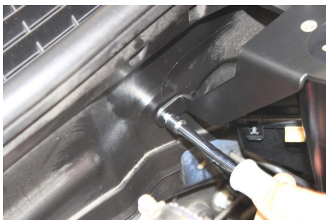
9. Align Catch Tank in vertical position and then using self tapping screw fix Tank bracket to plastic firewall. Note: Do not over tighten screw into plastic firewall.
