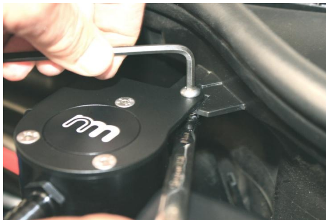
8. Vehicles without alarm switch start here. Remove air intake pipe or factory air box for easier access. Using M6x 16mm Button Head screw, washer and lock nut mount Catch Tank to top side of tab on plastic firewall.
