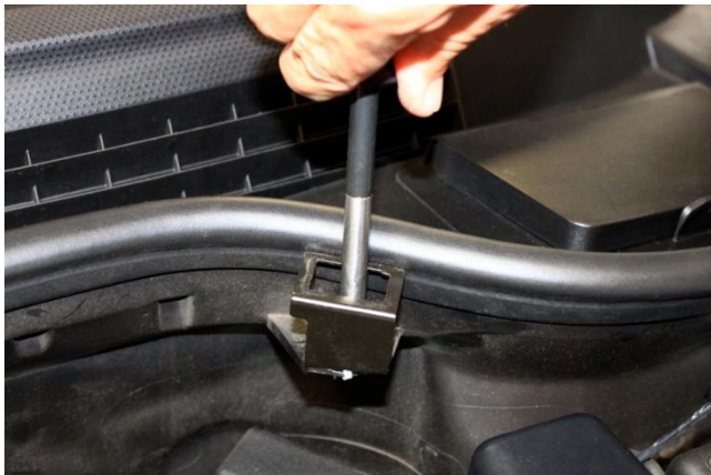
4. Remove bracket mounting screw with a T20 Torx.
