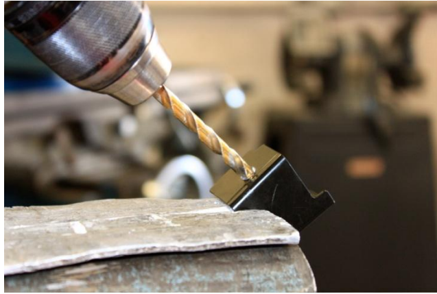
6. Enlarge bracket mount hole using 1/4" drill bit.
