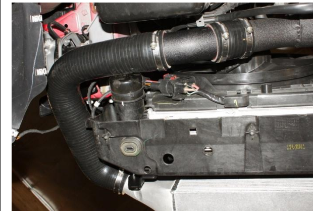
24. Install and tighten supplied driver side intercooler hose, 25° elbow tubing, 3" silicone hose and clamps as pictured. NOTE: Clamp screw at intercooler position to back side.
