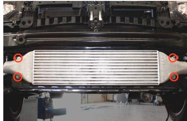
23. Mount intercooler core to vehicle using the supplied (4) 6mm hex flange nuts.
