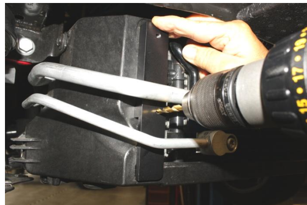
16. Attach both left and right side aluminum mounts into existing square holes in radiator core support, then lock down (make sure fully seated), using lower hole in mounting bracket drill through plastic core using 15/64" drill.
