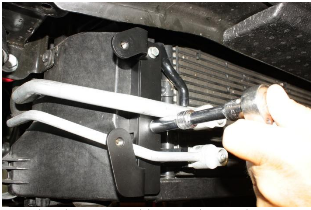
20. Right side mounting: slide up steel intercooler mounting bracket underneath A/C lines, then install with aluminum bracket to plastic core and tighten with supplied M6x16mm bolts (upper hole) and M6x35mm bolts (lower hole) using 10mm socket. Repeat mounting for left side.
