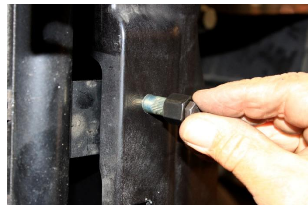
18. Install Nutsert using supplied setting tool (see separate tool instructions).
