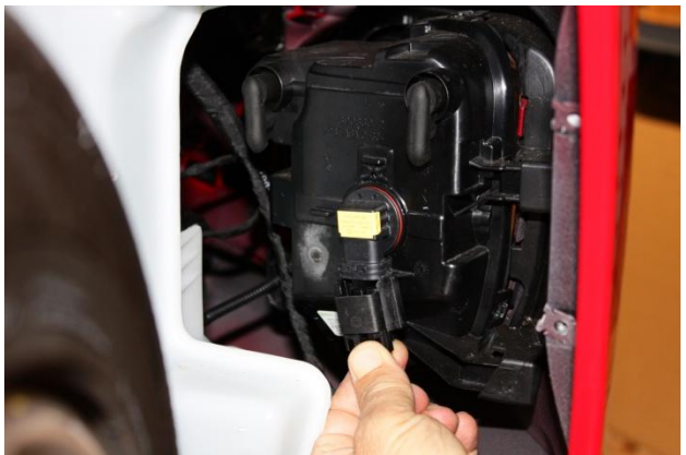
8. Before pulling front bumper completely off, disconnect both fog light connections.
