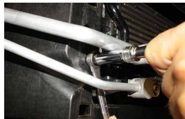
19. Hold body from turning with 14mm wrench then push and turn setting bolt with 10mm socket until Nutsert crimps firmly in hole. Remove tool.
