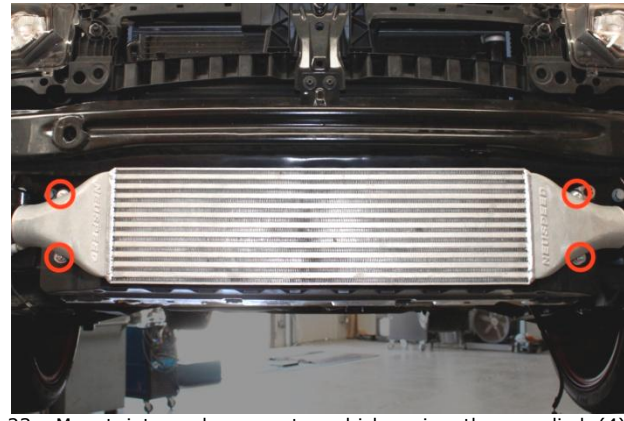
23. Mount intercooler core to vehicle using the supplied (4) 6mm hex flange nuts.
