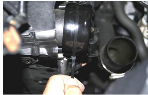
13. Using supplied cable ties, install black caps on inlet and outlet side of original intercooler.
