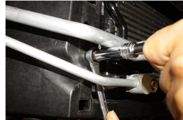
19. Hold body from turning with 14mm wrench then push and turn setting bolt with 10mm socket until Nutsert crimps firmly in hole. Remove tool.
