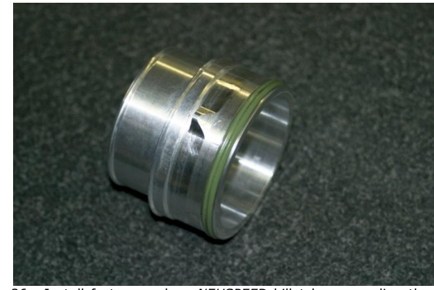
26. Install factory seal on NEUSPEED billet hose coupling then lightly oil.
