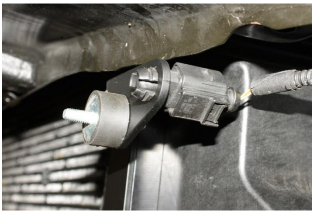
21. Install outside air temp sensor into hole in intercooler mount and install and tighten the 4 rubber isolators.
