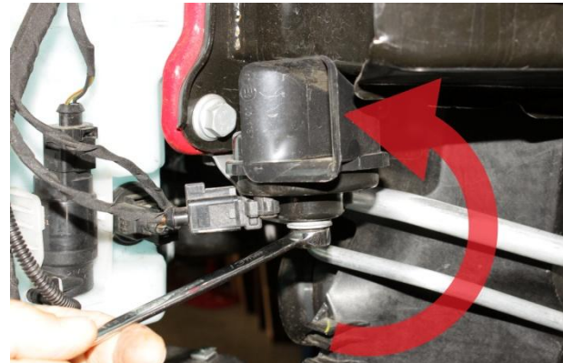
14. Using a 13mm wrench, unbolt right-side horn from its bracket and remount to the top-side, as pictured.
