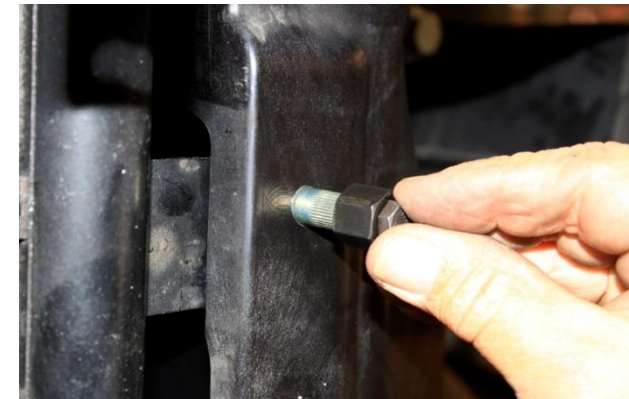
18. Install Nutsert using supplied setting tool (see separate tool instructions).
