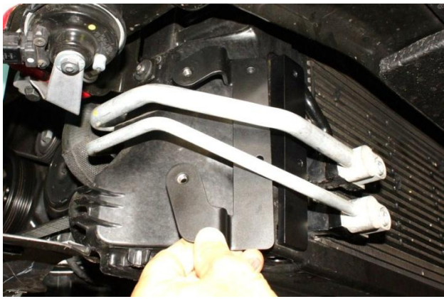
22. Both mounts shown installed.
