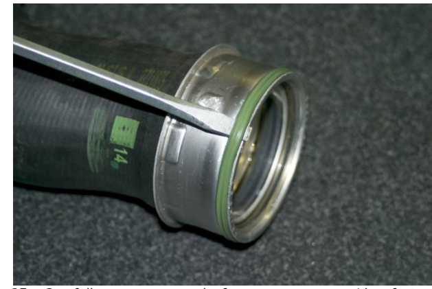
25. Carefully remove seal from passenger side factory intercooler hose.
