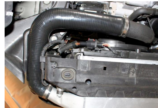
24. Install and tighten supplied driver side intercooler hose and clamps as pictured. NOTE: Clamp screw at intercooler position to back side.
