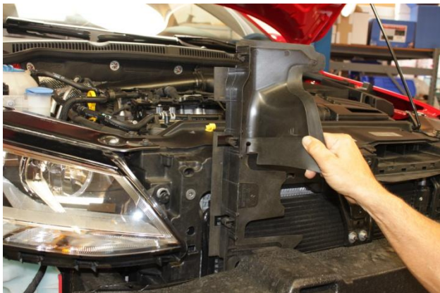
9. Unclip and remove the left and right side radiator air deflectors.
