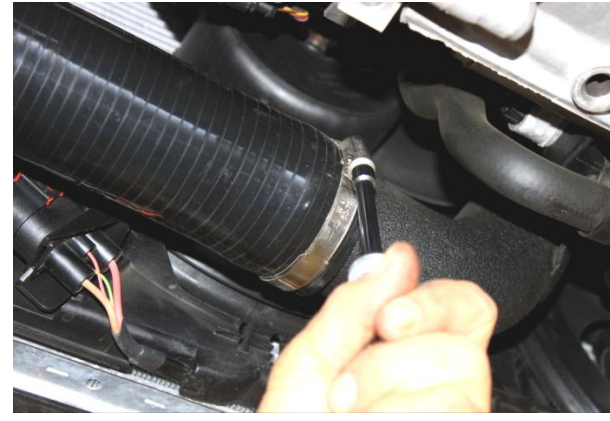
25. Carefully remove seal from passenger side factory intercooler hose.
