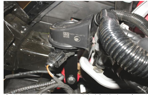
15. Using a 13mm wrench, unbolt left-side horn from its bracket. Remove OE bracket and using supplied "L" bracket, remount horn facing rearward and close to Air Pump if equipped as pictured.
