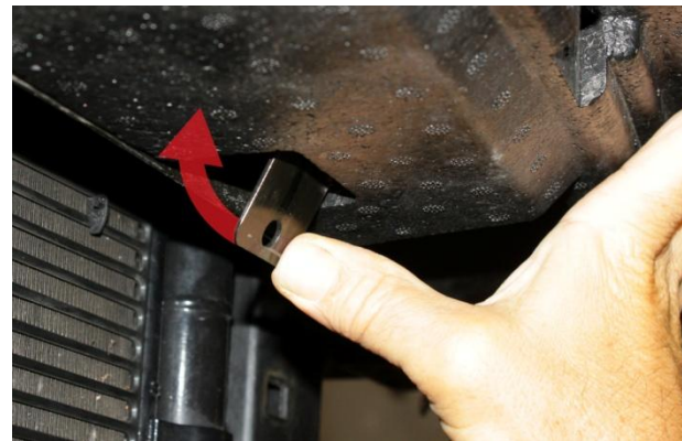
11. Bend metal temp sensor bracket backwards up horizontally.
