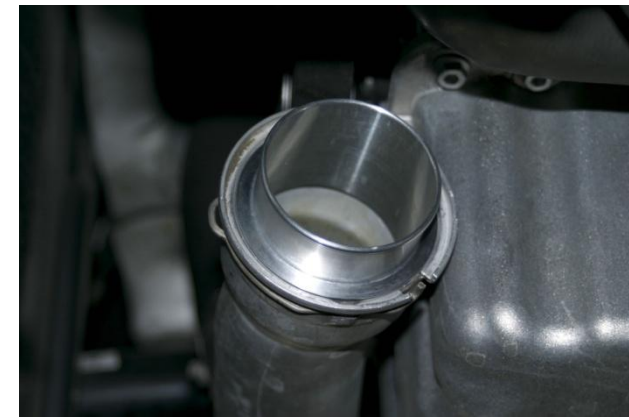
27. Install NEUSPEED billet hose coupling into turbo discharge pipe. Make sure clip locks onto billet adapter.
