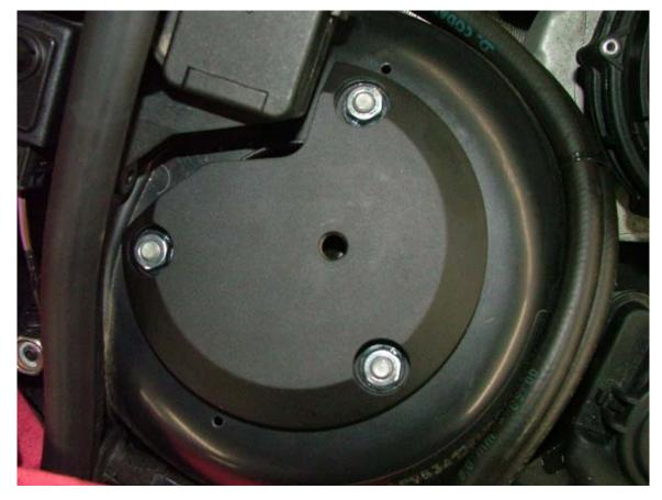
Install the right hand plate using the supplied stainless steel hardware.
