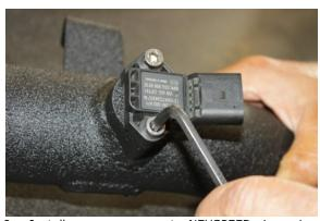
9. Install pressure sensor to *NEUSPEED* pipe using supplied M6 x 16mm bolts and tighten with a 5mm hex key wrench (note electrical connector direction as pictured).
