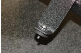
11. Install rubber grommet in *NEUSPEED* air charge pipe mounting bracket as pictured then install mounting screw.
