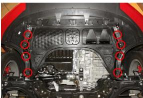
Raise the front of vehicle and support with jack stand(s) under lifting points. **NEVER WORK** ON A VEHICLE ONLY SUPPORTED BY A **JACK.** Remove lower engine splash pan, (8) T25 Torx screws. **NOTE:** GLI shown in picture, other models may vary.
