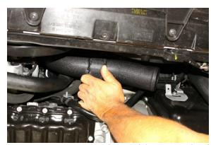
12. Use WD-40 or equivalent to lubricate inside of upper rubber hose and generously loosen hose clamp to ease pipe installation. Install NEUSPEED pipe from underneath and insert into upper rubber hose.
