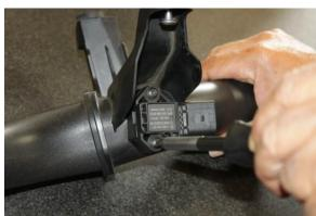
8. Using a T20 Torx remove pressure sensor from original pipe.
