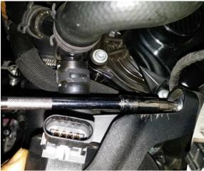
5. Unbolt upper air charge pipe mount screw using a T30 Torx.
