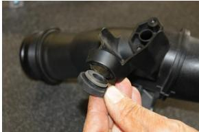
10. Pull out one of the mounting screws and rubber grommet from original pipe.
