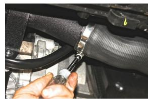
15. Use WD-40 or equivalent to lubricate inside of lower rubber hose and generously loosen hose clamp to ease pipe installation. Attach lower rubber hose to *NEUSPEED* pipe. Check alignment of *NEUSPEED* pipe and tighten lower hose clamp.
