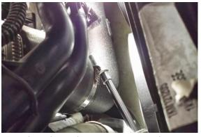
16. Tighten hose clamp at upper air charge pipe connection.
