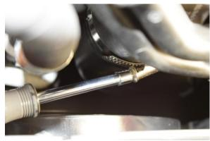
1. Loosen hose clamp with a 7mm Nutdriver or screwdriver at top of plastic air charge pipe to rubber hose located below throttle body.
