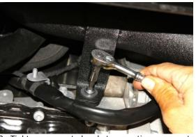
13. Tighten support bracket mounting screw to original lower mounting hole in engine using T30 Torx.
