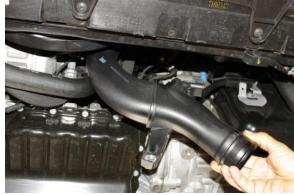
7. Rotate pipe to break free from upper rubber hose, and then pull out from underneath vehicle to remove.
