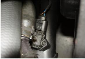
4. Reach to top side of air charge pipe and disconnect boost pressure sensor. Squeeze tab then disconnect electrical connector.
