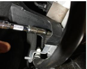
Unbolt lower air charge pipe mounting screw using a T30 Torx.
