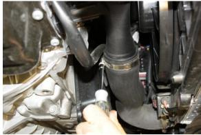
3. Loosen hose clamp using a 7mm Nutdriver or screwdriver at lower air charge pipe connection and disconnect from rubber hose.
