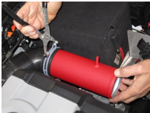
16. Install intake pipe with port closer to the front and positioned at 1 o'clock.
