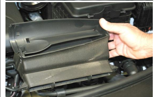
9. Remove air intake duct at radiator support (2) T25 Torx, one on each side.
