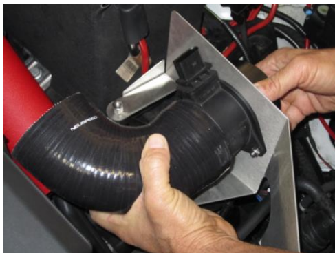
16. Install intake pipe with port closer to the front and positioned at 1 o'clock.
