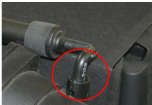
2. Disconnect vacuum hose from air filter box lid.
