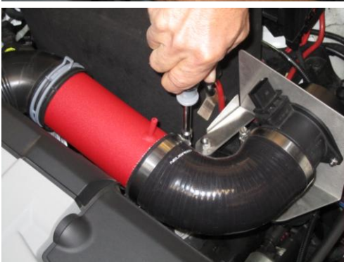
17. Install 90° silicone hose onto MAF. NOTE: Use silicone spray to ease install. Slide the two supplied #48 hose clamps onto silicone hose and then connect to intake pipe. Now position clamps and tighten.
