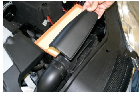
6. Remove cover at intake duct.
