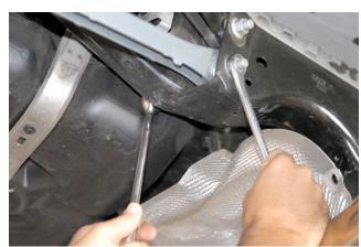
Unbolt and remove inner control arm bolt using 18mm socket and wrench.
