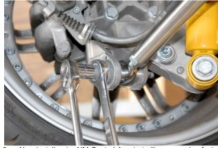
Now install outer NM Control Arm to trailing arm using factory bolt and adjusting plate. Line-up previous made pen mark before tightening. Torque both inner and outer control arm bolts to 100Nm (74ft.lbs).
