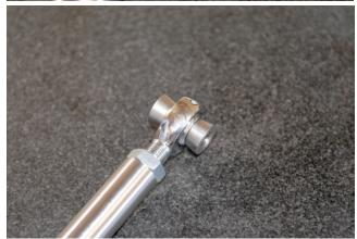
Install supplied stainless steel spacers into ball joints. The NM Control Arms have been pre-set to the factory length of 20 15/16".
