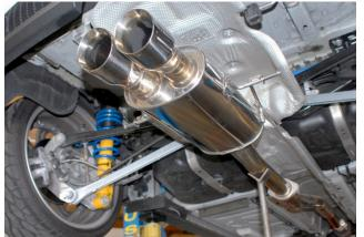
Spray WD-40 or equivalent on rear muffler exhaust hanger pins. Support exhaust while using a screwdriver to pry off rubber exhaust hangers from muffler.
