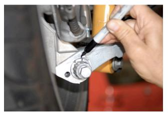
Mark existing location of factory adjusting plate to trailing arm on outer control arm bolt with marking pen.
