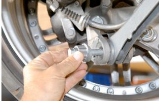
Unbolt and remove outer control arm bolt and adjusting plate using a 16mm socket, then remove control arm.
