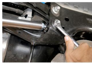
Install NM Control Arm into inner mount. NOTE: Adjusting flats on NM bar goes outward.
