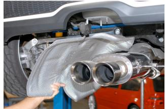
Lower and support exhaust system just enough to unbolt and remove rear muffler heat shield from vehicle, (3)10mm hex nuts and (2)10mm hex bolts.
