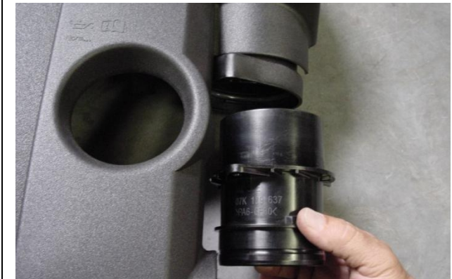
8. Remove (2) Phillips screws that mount the air box inlet adapter to engine cover and separate.
