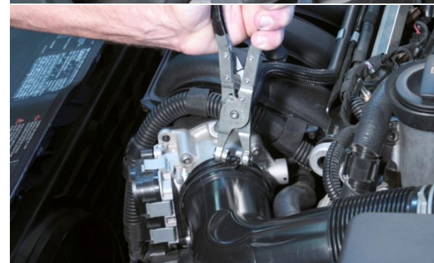
5. Disconnect Secondary Air Injection hose (if equipped) and crankcase ventilation hose from intake air duct, squeeze collar to release locking tabs. Release spring clamp at throttle body and remove intake air duct.
