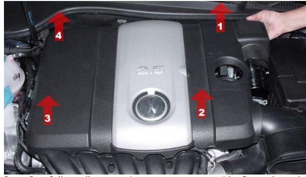
3. Carefully pull up engine cover on one side first, then the other side. To ease removal, spray WD-40 or equivalent on rubber mounts underneath cover. NOTE: If rubber grommets remain on ball pin mounts, remove and replace underneath cover.
