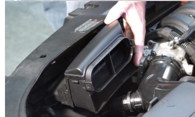
4. Remove air intake connection from front core support by removing (2) T25 Torx screws on each side.
