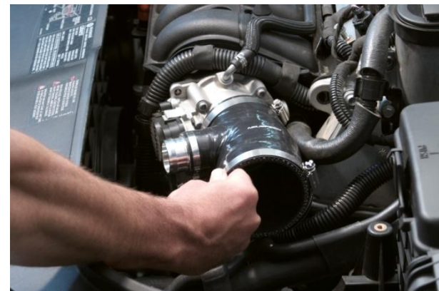
6. Loosely attach silicone hose onto throttle body with #48 hose clamp and #52 hose clamp on opposite side.
