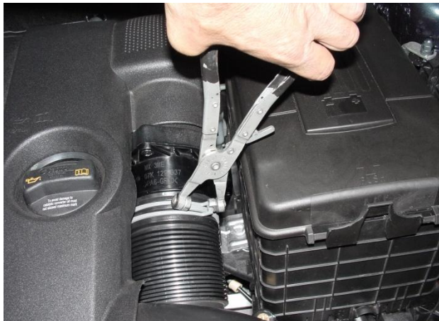
2. Disconnect intake hose from air box inlet adapter (dummy MAF) using spring clamp pliers or equivalent.
