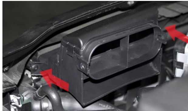
3. Carefully pull up engine cover on one side first, then the other side. To ease removal, spray WD-40 or equivalent on rubber mounts underneath cover. NOTE: If rubber grommets remain on ball pin mounts, remove and replace underneath cover.
