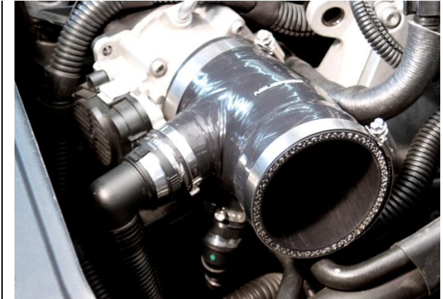
7. Connect crankcase ventilation hose and Secondary Air Injection hose to billet fittings on silicone hose. NOTE: For vehicles not equipped with Secondary Air Injection use supplied vinyl cap and wire tie on billet fitting.
