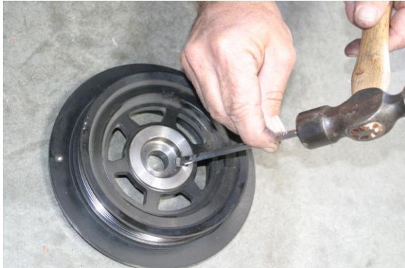
9. With a hammer and chisel, carefully remove key from crankshaft pulley. NOTE: Do not lose or destroy key, not available separately from VW Parts.
