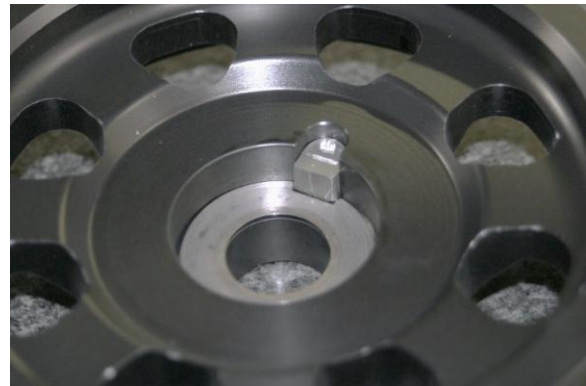
12. Install shim washer onto back side of pulley.
