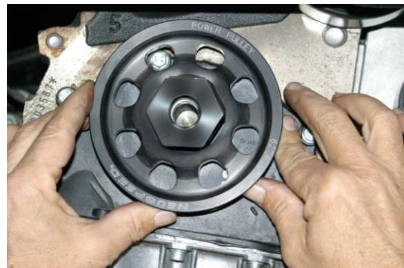
13. Position pulley on crankshaft and align key to keyway. Gently press pulley onto shaft. If pulley does not slide on shaft easily, remove and check for burrs or corrosion. If any burrs or corrosion exists, remove as necessary. Use of excessive force to install the pulley will damage both the pulley and the crankshaft and will void warranty.
