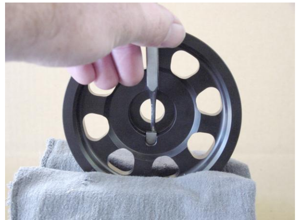
11. Install key in keyway of NEUSPEED crankshaft pulley and gently tap into position if required.
