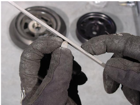
10. Remove any burrs from key with a file.
