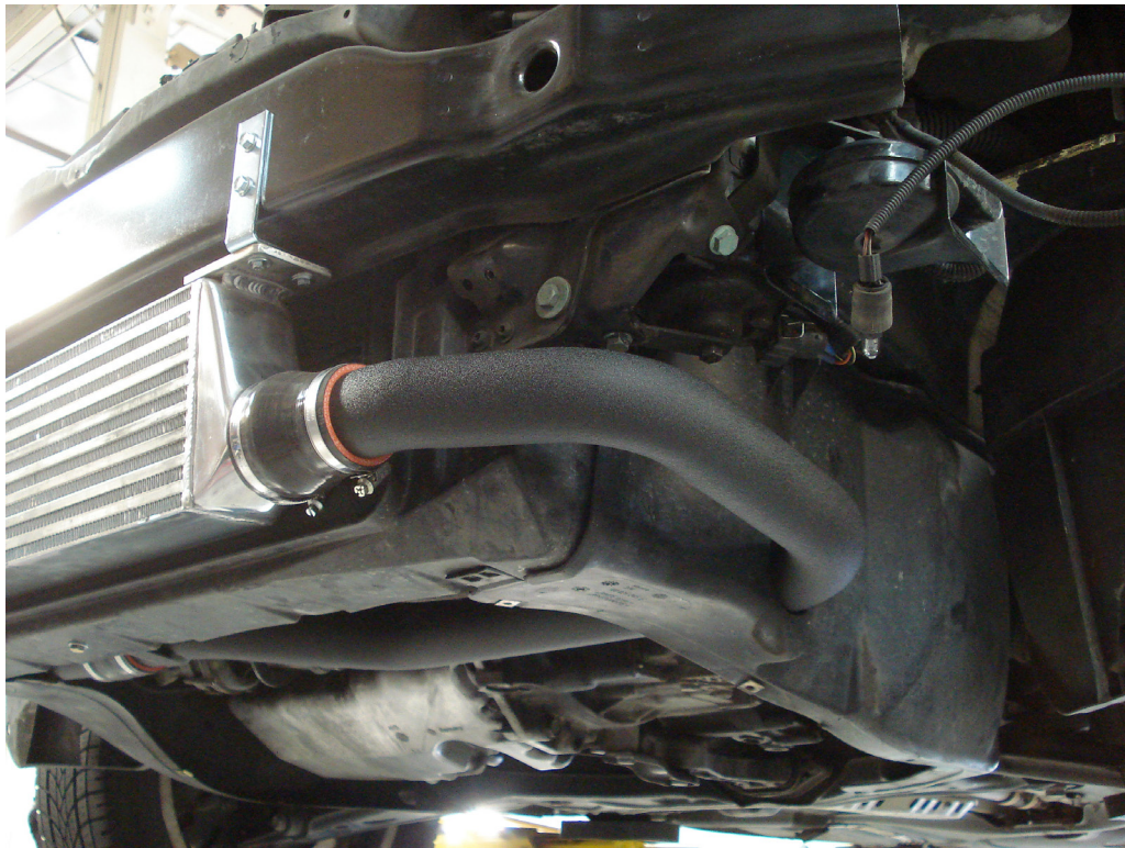
Step 20. Install silicone hose on both sides of intercooler and route drivers side intercooler pipe through drivers side engine cover as shown.
