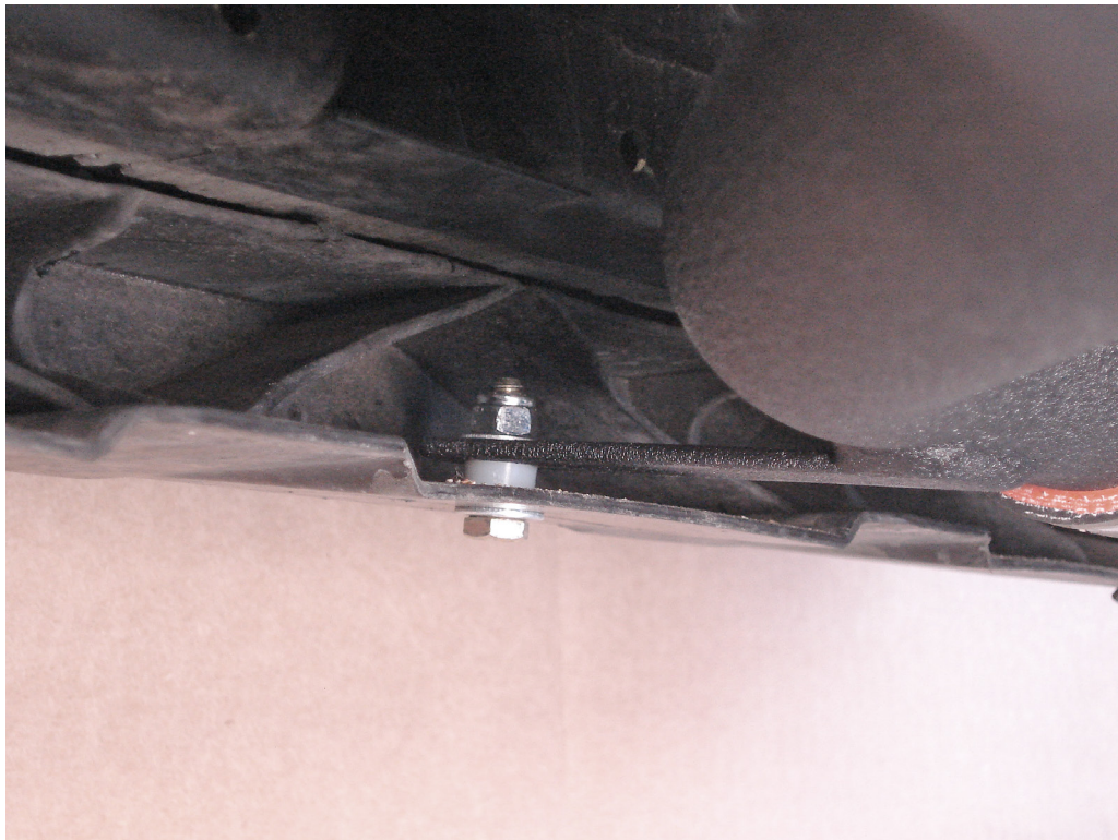
Step 22. Intercooler mounting bracket properly installed with supplied hardware.
