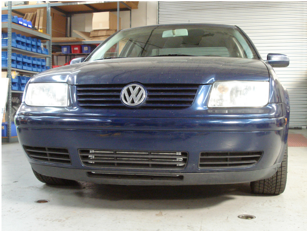
Step 28. Installation of intercooler complete.
