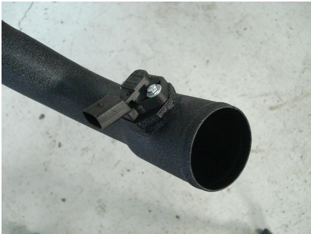
Step 10. Re-Install the factory MAP sensor onto the Euro Sport intercooler tube using supplied hardware (two bolts and washers) and gasket.
